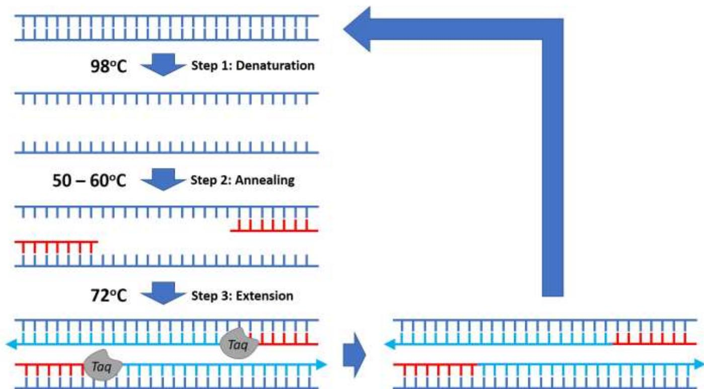
Each PCR cycle, the region flanked by the primers is doubled (if the reaction is 100% efficient). Thus, after the 1<sup>st</sup> cycle, there is twice as much, after 2 cycles, 4X, after 3 cycles, 8X, and so on. After about 30 cycles, you can generate over a billion molecules of DNA from a single copy of the template!
