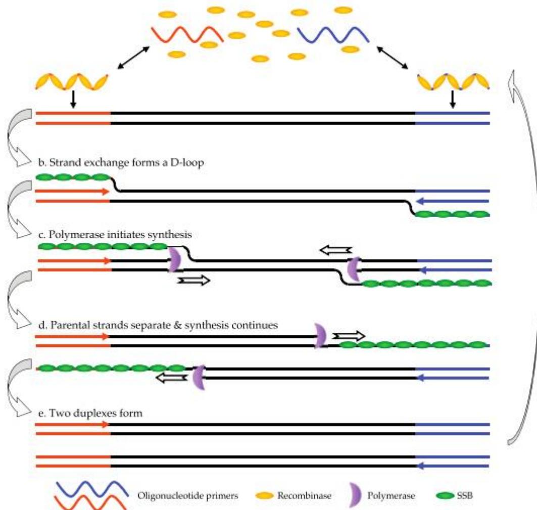
At room temperature and constant temperature, the recombinase and primers form a protein / single stranded nucleotide complex rec / ssDNA, which invades the double stranded DNA template with the help of helper protein and single stranded binding protein SSB.
