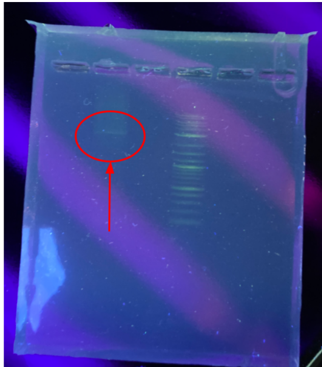
Figure 1. Successful gel results of PhoA Colony PCR. Well 2 contain the PhoA DNA, and well 4 contains the standardized DNA ladder (4/26/21).
