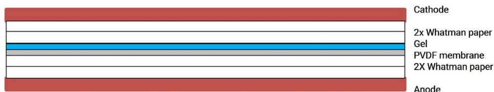
Figure 2: Set-up of the blotting sandwich for western blotting. We used a Semi-Dry blotting technique. Therefore, the PVDF membrane was activated in methanol and two layers of Whatman paper, preequilibrated in blotting buffer, were placed above and under gel or membrane, respectively.
