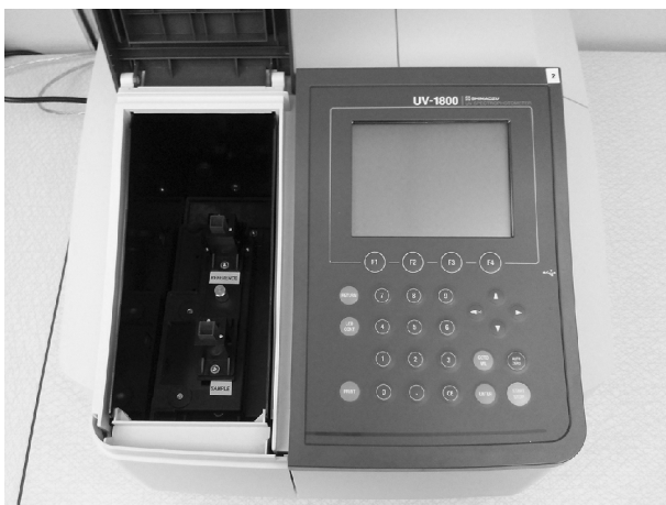
Fig. 13 UV-visible spectrophotometer containing 1 mL sample and reference cuvettes.
