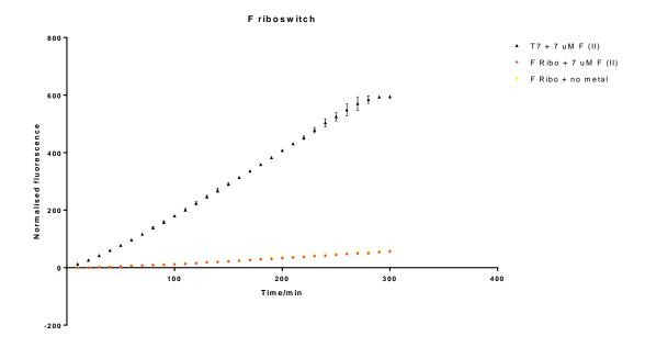
No difference observed for the fluorescence of reactions with or without the presence of metal ions. Indeed, the riboswitch dependent termination uses the mechanism of Rho dependent termination, which cannot stop T7 Rpol transcription. Another construct using Anderson promoter has been designed.
