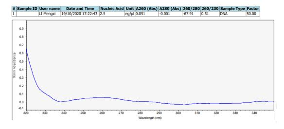
According to calculation, the total amount of DNA added into the digestion system is 528ng. The concentration in 50 ul system should be 10.5 ng/ul. Which is 5 times higher than the measured concentration. Could be the problem with the blank (EB was used as blank), or DNA degradation happens.
