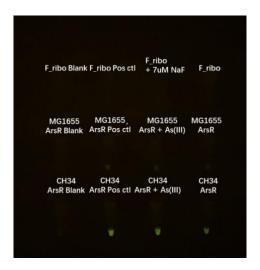
No fluorescence for the riboswitch positive control is because T7 RNA polymerase was forgotten to add
