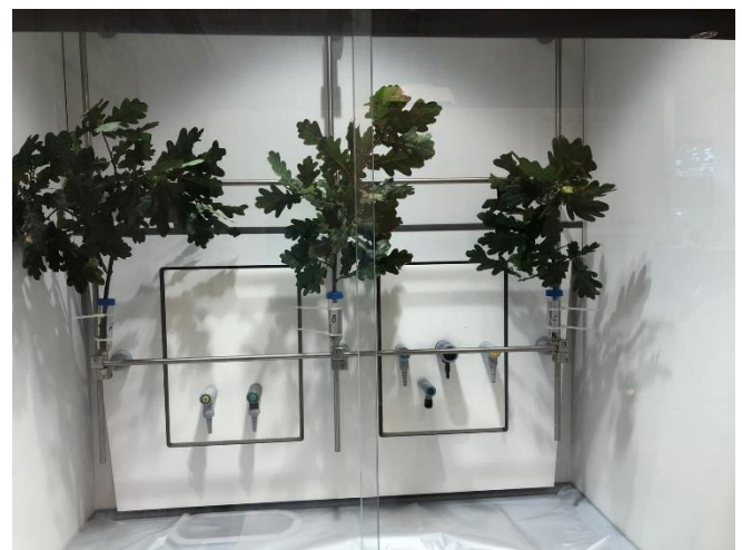
Figure 4: Experiment if the pesticide sticks to the trees. Testing it on oak branches in the laboratory.
