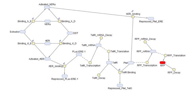
Here, we are modelling another design that will lead to a biosensor that can discriminate between DDT and estrogen (or other xenoestrogens). In this case, we would need to optimize the circuit based on the differential binding affinities of estrogen receptors from different species (such as human and rainbow trout) to estradiol or DDT.
