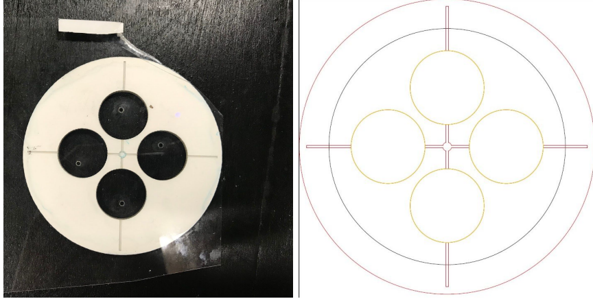
Figure 25. Left: the Chip tested, Right: Laser cut vector file
