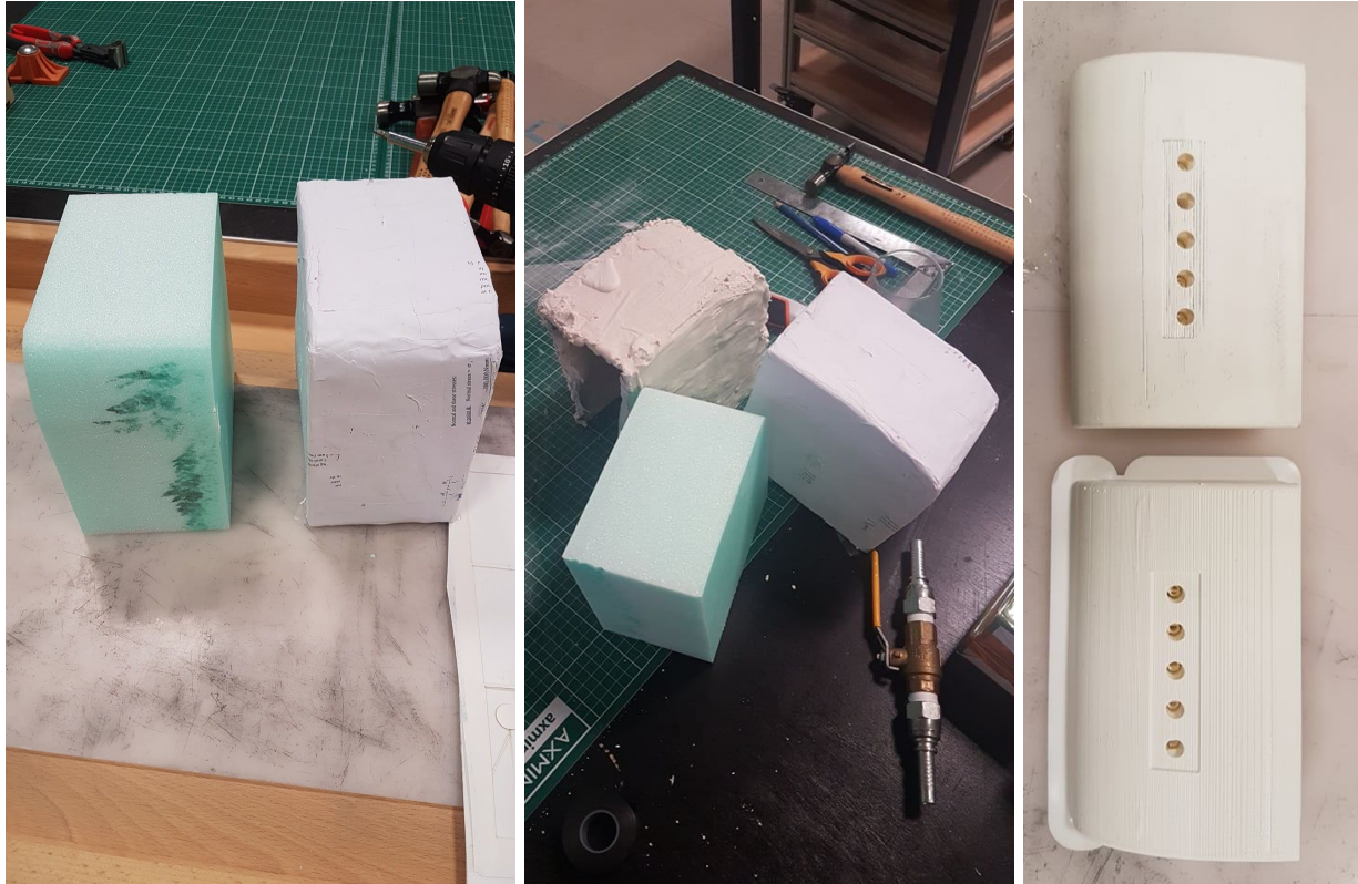
Figure 9,10,11: As part of the process we experimented with a series of materials, but 3D printing and sanding PLA ended up being the best solution.
