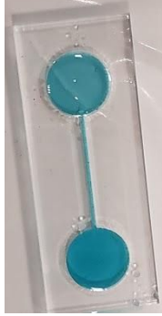
Figure 6: Testing acrylic flow on a hydrophilic floor
