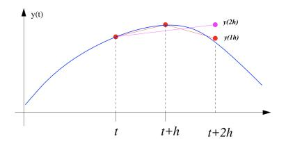
$\begin{cases} The calculator is too precise and the step size h should be reduced to gain calculation time. if <math>h < h' \\ The error exceeds h'\delta$ , and the step size should be reduced to gain precision otherwise
