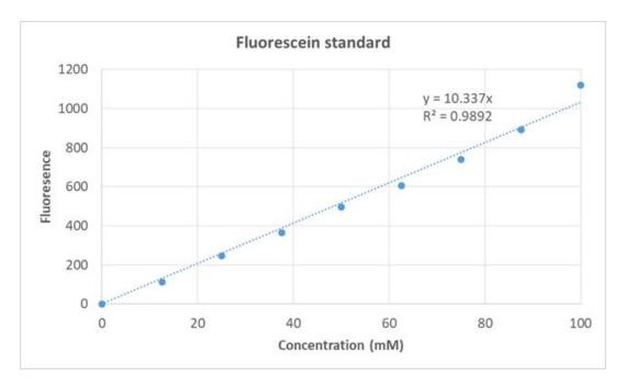
Fluorescein provided by iGEM was used a standard for fluorescence measurement. The near linear response of fluorescence signal with increasing concentrations of fluorescein (0 - 100 mM) shows that our instrument (Odyssey FC) can measure fluorescence signals between 0 and 1000 reliably.
