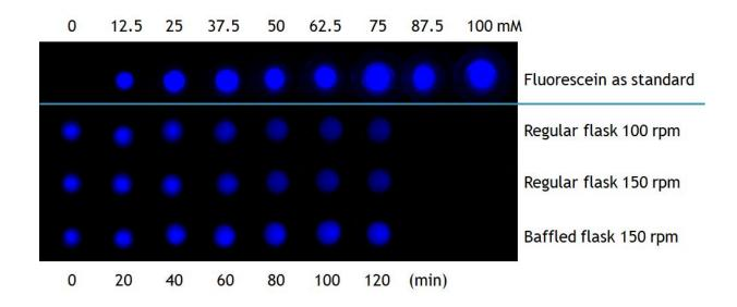
Making calibration curve using fluorescein standard from iGEM
