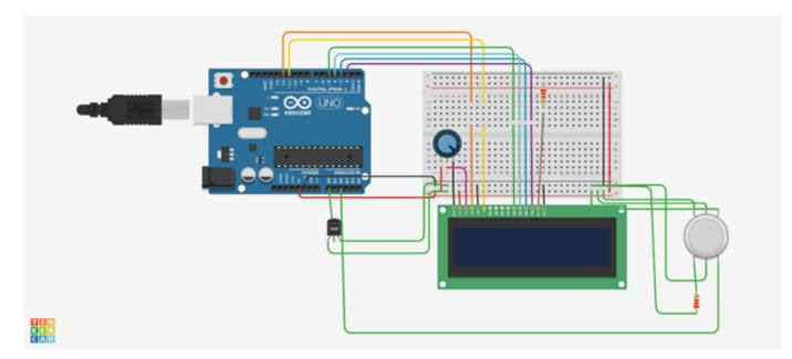
You should weld the cables in the Universal Plate using the 38W solder (They generally come with the Arduino Unit, a 10x10 unit should be enough) and then connect them in the Arduino following the image above, or as you prefer. It should be very simple to master welders, but a bit challenging for novices. We recommend doing things one at a time, and testing them after every successful welding, even if it is a lot slower, it will be the safest approach. And as always, safety should come first.
