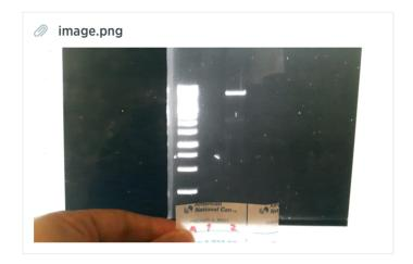
PCR only worked with BB2, so I proceeded with BB2. cloning was done, controll was lysed bacteria, positive was arac3 plasmid
