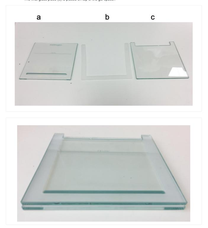
2. Set up the glass casting apparatus.
