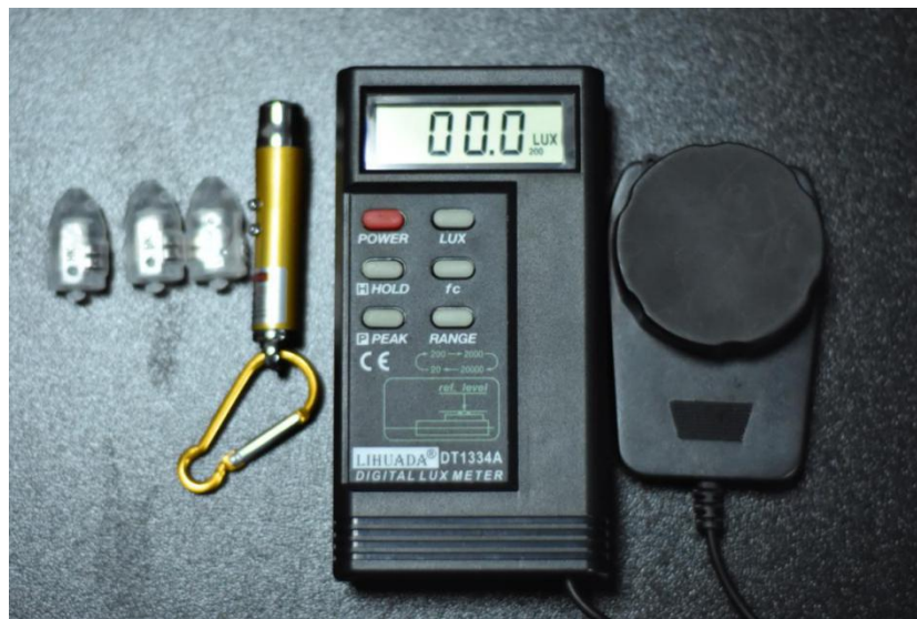
Figure 2. Light sources and illuminance meter
