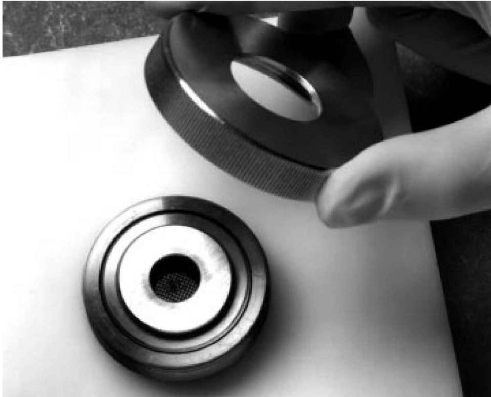
Fig. 4.10. Removal / replacement of macrocarrier cover lid with assembled fixed nest. Macrocarrier holder (with macrocarrier properly inserted) is inverted and placed atop fixed nest.
