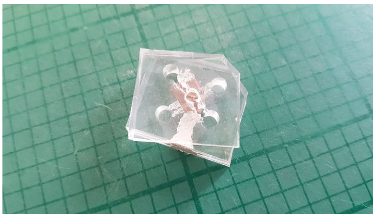
FIGURE 4 – Assembled vertical chip with gold-coated membrane filter
