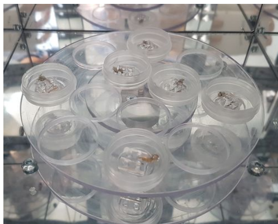
FIGURE 7 – Dishes and their lid in UV curing unit
