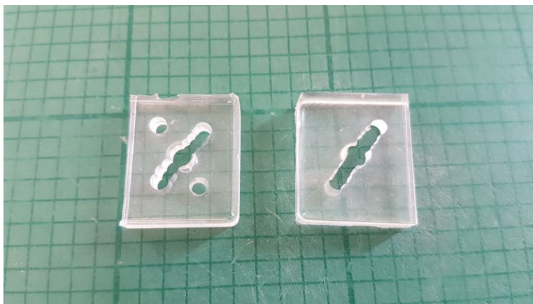
FIGURE 3 – Two halves of PDMS layer. Left : upper layer. Right : bottom layer
