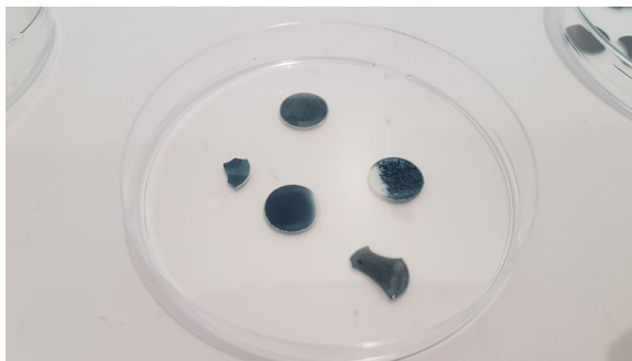
FIGURE 11 – PEDOT :Ts coated membranes
