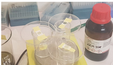
FIGURE 10 – Vapor phase polymerization of PEDOT :Ts
