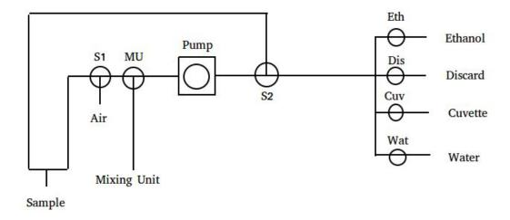
The sample part, the mixing unit part Cuvette will be explained further. The discard, Ethanol and Water are just beakers corresponding to their respective contents.
