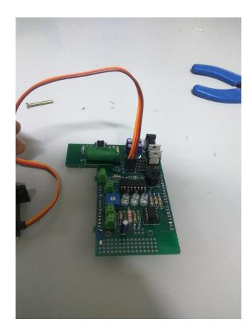
Attach the PCB to the Arduino, and complete the circuitry according to the schematics.
