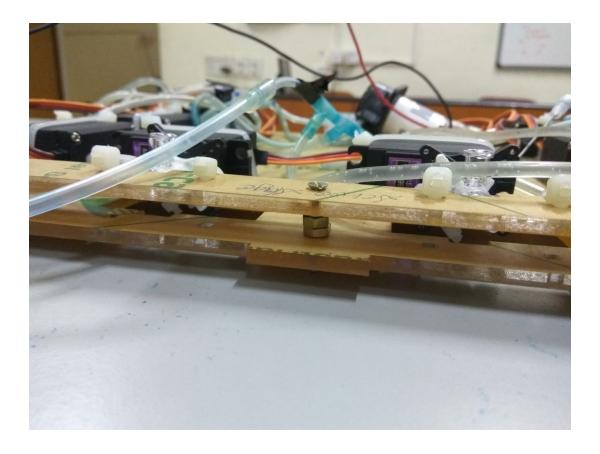
Attach the three-way stopcocks to the corresponding grooves on the top panel of the Case using zip ties. We will be using zip ties to attach more things soon.
