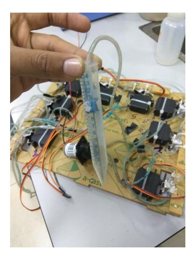
The sampling tube is made from a tube perpendicular pierced by a syringe needle. This is the part that will go inside the shaker.
