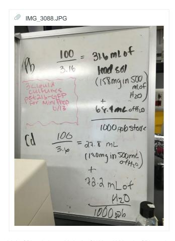
31.6 of Pb solution + 68.4 mL of H20 = 1000 ppb of Pb stock 27.8 mL of Cd solution + 72.2 mL of H20 = 1000 ppb of Pb stock Continued to follow DIY Lead Assay Protocol
