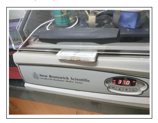
You should wrap the cable around something in the shaking platform so that the USB port on the device does not have to bear any strain.
