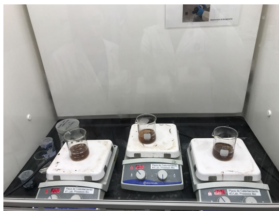
Figure 8. Heated bagasse samples with acid detergent at 200°C
