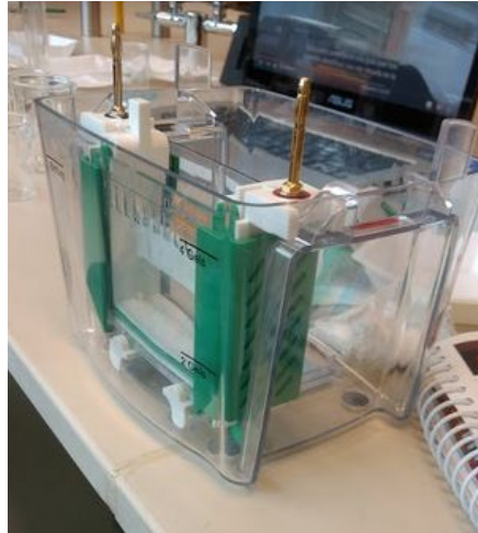
Completed gel inside the electrophoresis chamber, before the addition of the running buffer.
