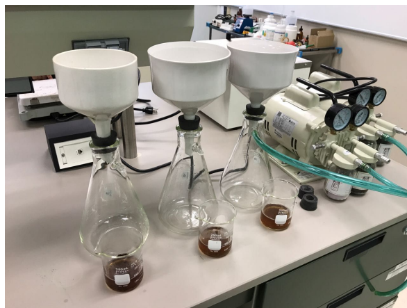
Figure 9. Filtration system of FND acid solution
