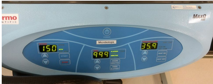
Conditions of the thermoshaker for the incubation of the P. putida kt2440.
