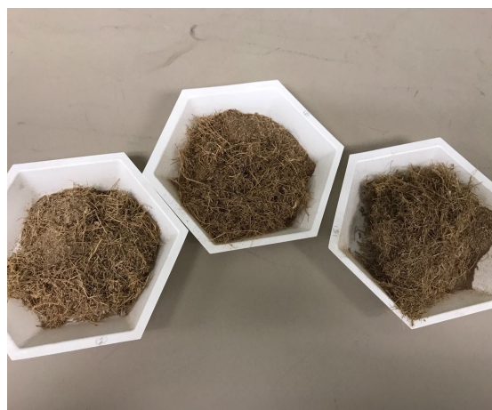
Figure 5. Dried and milled bagasse set after alkaline treatment
