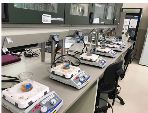
Figure 6. Heated bagasse samples with neutral detergent at 300°C
