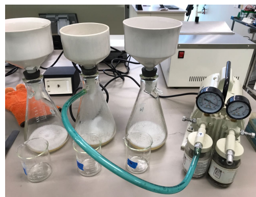
Figure 7. Filtration system of FAD solution
