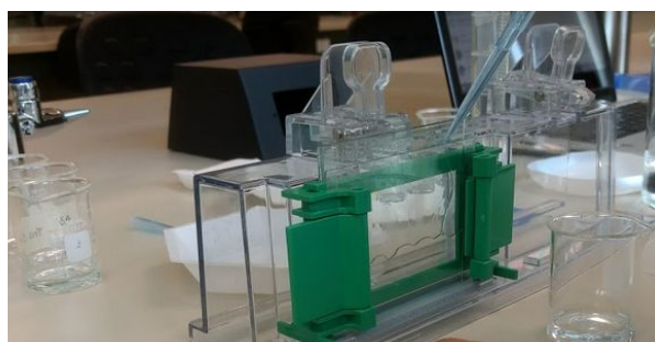
Addition of the stacking gel between the glasses.
