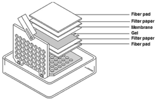
*Note: Set up the sandwich in a plastic tray filled with transfer buffer. Ensure that any bubbles on the membrane is removed using the roller brush.*
