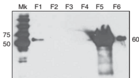
Figure 6 | Western blot analysis showing the IMAC purification steps of a chimeric Flag/MaSp 2 recombinant protein. The 60-kDa His-tagged A4S8 8 recombinant protein was detected using the 6× His mAb–HRP conjugate. Mk: molecular weight marker Precision Plus Protein Standard Dual color; F1–6: IMAC collected fractions—F1: unbound proteins; F2–4: wash 1 (20 mM imidazole), wash 2 (40 mM imidazole), wash 3 (50 mM imidazole), respectively; F5: elution fraction (250 mM imidazole); F6: strip fraction. The recombinant protein is highly concentrated in the elution fraction (F5) and residual in the strip fraction (F6). The numbers indicate the molecular weights in kDa.
