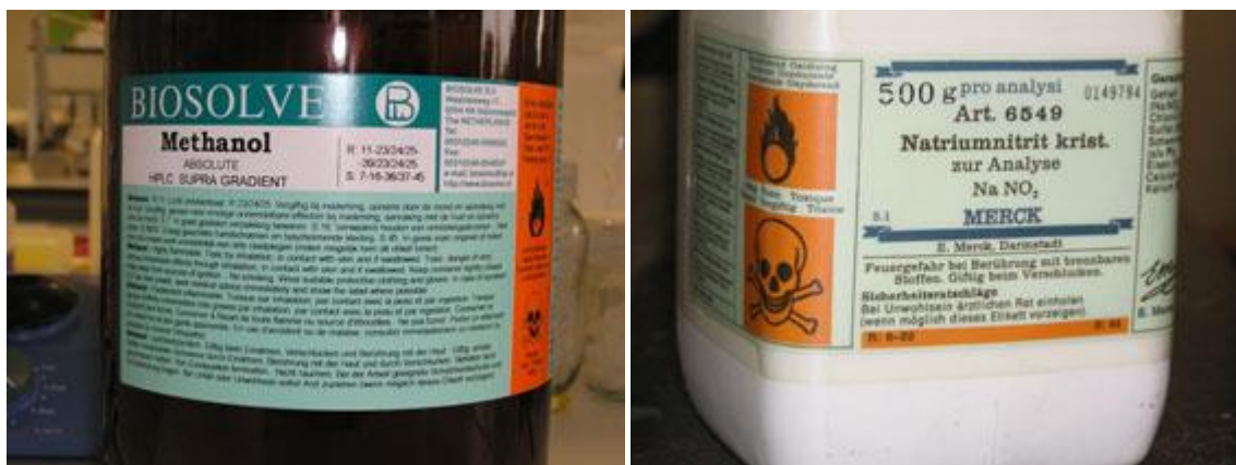
Labels on chemical packings with 'R' and 'S' phrases and danger symbols
