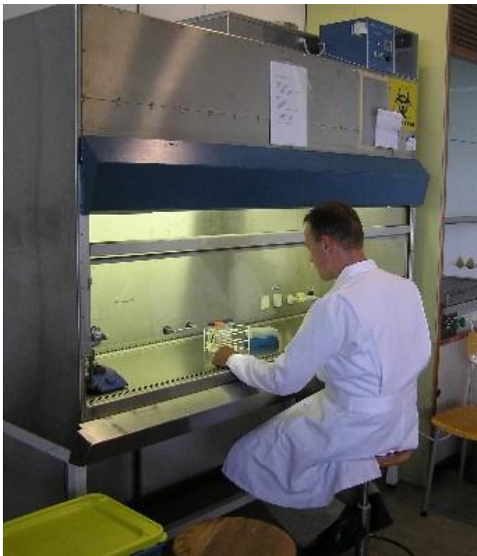
A safety cabinet is mandatory if you are working with class 2 biological agents
