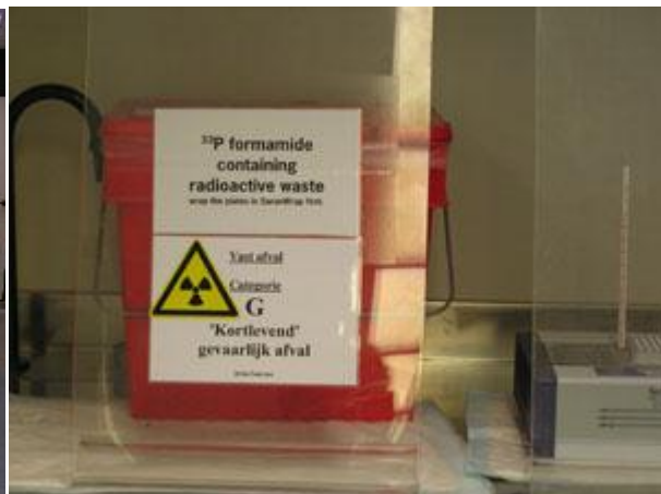
Waste container for "short-life" radioactive waste
