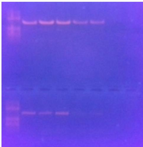
50 µL was loaded in each well on a 1 % agarose gel. Ladder: red. The upper line is the PCR result for this protocol. There appeared band in all wells around 2000 bp. The bands were cut out and purified from gel.
