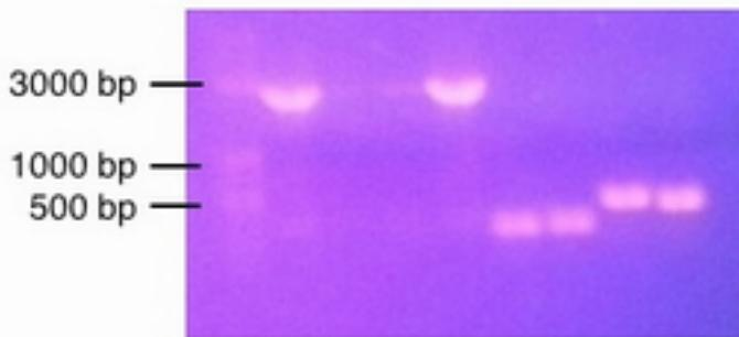
Well 1-4 contains colony PCR of cells transformed with dxs (E.coli) in pSB1C3. Bands around 2200 bp appeared in all four wells, but the strongest bands is in well 1 and 4 (colony 1 and 4).
