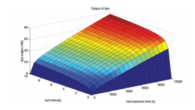
We see that the value depends on both intensity and exposure time, but the upper limit with respect to the intensity is reached quite quickly. The output seems to depend linearly on the exposure time and does not seem to be anywhere near reaching a limit.
