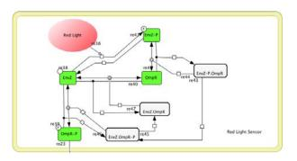
If the binding mechanics for the OmpR promoter are of interest, one should consult the paper by Yoshida [3]. They have not been integrated in this model, see the guide for details on how to do that.
