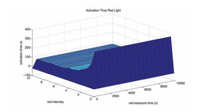
We see that the activation time only depends on the intensity of the light, not on the exposure time which should coincide with the real world behavior.
